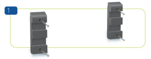
Drill holes through the end cap retainer and fix to the wall using the appropriate fixings leaving 35mm from your start point to allow for the end cap.
