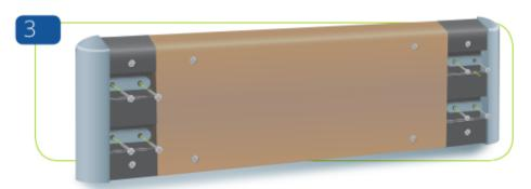
Fix end caps onto retainers using screws - maximum length 25mm
