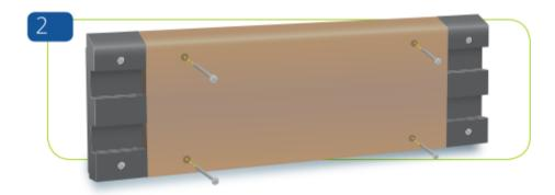
Cut the MDF core to required length. Drill holes at maximum 800mm centres, starting 50mm from either end. Finish the MDF core run with another end retainer.
