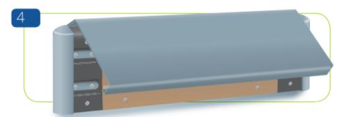
Measure between end caps and cut cover to length - make a joint if necessary. Clip on profle from the upper part of the MDF core by pushing downwards
