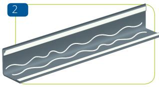
Apply two beads of construction approved adhesive near the corner of the guard.
