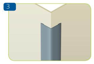
Apply to the wall and ensure corner guard is securely stuck by applying firm, even pressure.
