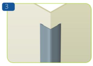
Apply to the wall and ensure corner guard is securely stuck by applying firm, even pressure.
