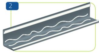
Apply two beads of construction approved adhesive near the corner of the guard.
