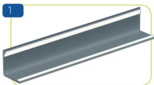
Cut the corner guard to the correct length and ensure the back is clean. Apply one strip of double sided tape 2mm from each edge.
