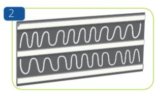
Make sure wall is clean. Apply construction approved adhesive between the bands of tape. Remove the double sided tape backing.
