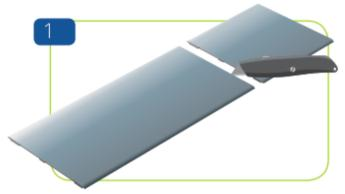
Measure the wall then cut the rub rail to the correct length using a sharp Stanley knife.
