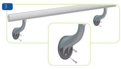
Fix brackets to the wall using construction approved fxings making sure the brackets are level.
