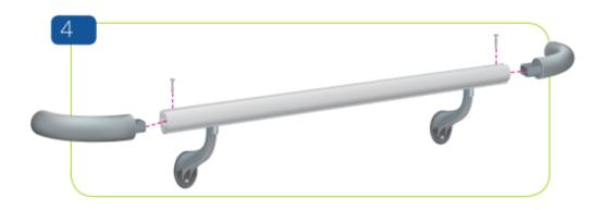
Attach the endcaps to either end of the aluminium rail and fx with selftapping screws.
