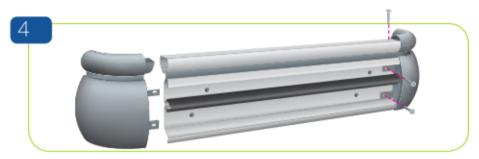
Insert sheet strip and two-part endcaps onto aluminium retainer..... and secure with screws.
