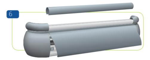
Measure between endcaps and cut handrail and bumper covers to length. Clip on handrail and bumper covers.
