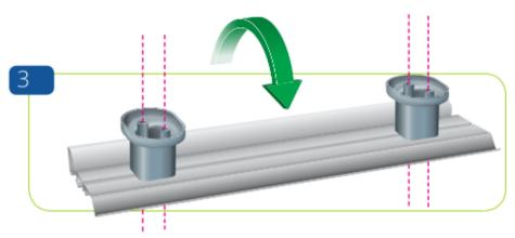
Using a 7mm drill bit, drill holes through the aluminium retainer from the back using the attached mounting brackets as guides.
