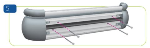
Hold the rail at the required height and use the retainer as a template to mark the fxing points. Screw the rail to the wall using construction approved fxing methods.
