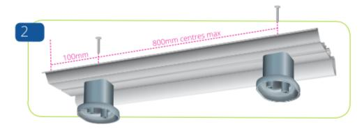
Fix the mounting brackets to the aluminium retainer using short self-drill screws. Begin 100mm from either end with maximum 800mm centres thereafter.
