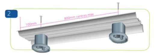
Fix the mounting brackets to the aluminium retainer using short self-drill screws. Begin 100mm from either end with maximum 800mm centres thereafter
