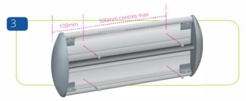
Starting at 100mm from each end, drill holes through the retainer at a maximum of 500mm centers, mark fixings on the wall using the drilled retainer as a template. Use construction approved fixings to affix retainer to the wall.
