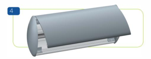
Measure between endcaps and cut the cover to length. Clip on the cover starting from the top and pushing downwards ensuring a snug ft.
