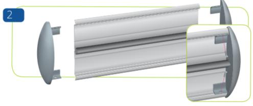
Insert and attach endcaps using 15mm screws
