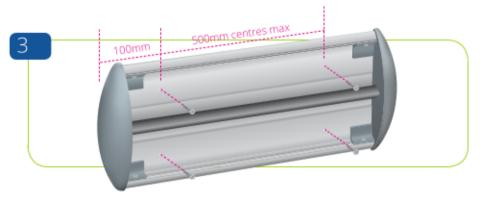
Starting at 100mm from each end, drill holes through the retainer at a maximum of 500mm centres. Mark fxing points on the wall using the drilled retainer as a template. Use construction approved fxings to affx retainer to the wall.
