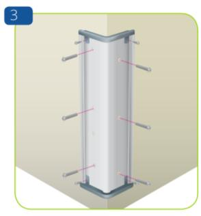
Fix the retainer to the wall with construction approved fxings. Fasten endcaps using short self-drilling screws.
