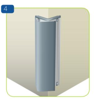
Clip on the cover, starting from one side, pushing the opposite direction and ensuring a snug ft. (Endcaps can be adjusted to align with the cover).
