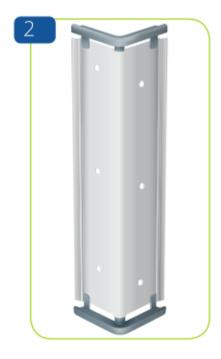
Insert top and bottom endcaps onto the aluminium retainer
