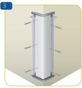
Fix the retainer to the wall with construction approved fxings. Fasten endcaps using short self-drilling screws.
