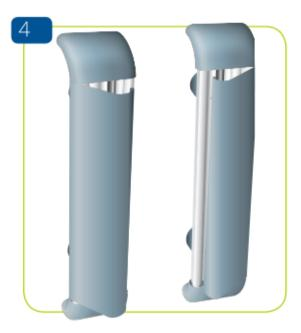
Attach the cover starting from the outside edge and pushing inwards to ensure a snug fit.
