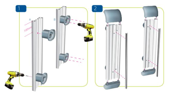
A. Fix the brackets onto the back of the aluminium retainer using short self-tapping screws through the front of the retainer nd into the bracket itself – brackets being attached 100mm from each end.
