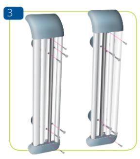
Mark fixing points on the wall using the drilled retainer as a template. Fix the retainer onto the wall with construction approved fixings.
