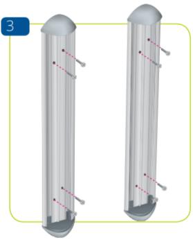
Mark fixing points on the wall using the drilled retainer as a template. Fix the retainer onto the wall with construction approved fixings.
