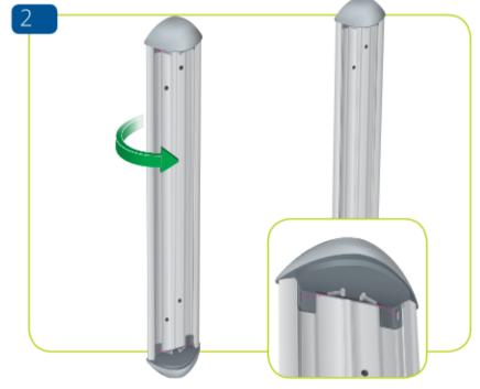
Hold a 10mm spacer to the back of the retainers and drill holes through the retainer using the spacer as a guide.
