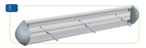
Mark the fixing points on the wall using the drilled retainer as a tempate. Ensure a spacer bracket is aligned to each fixing point and screw retainer to the wall using construction approved fixings.
