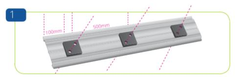
Cut the aluminium retainer to the correct length allowing for an endcap at either end. Hold a 10mm spacer bracket to the reverse of the retainer and starting 100mm from either end and with a maximum of 500mm centres (spaced evenly) drill through the aluminium retainer to create fixing holes.
