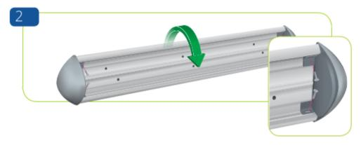
Turn over and attach endcaps to the retainer using screws of a maximum length 15mm.
